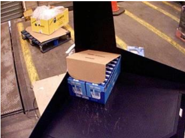
The flap used to secure retail units is loose.
