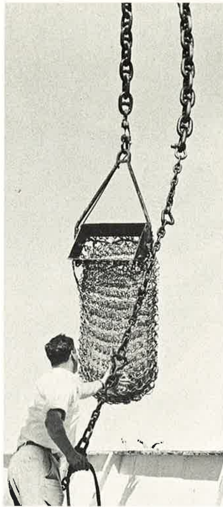
This is a rock dredge used by the crew of CSS "Hudson" to scour the ocean bottom for geological specimens.
